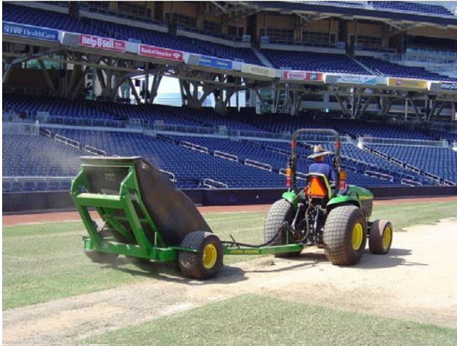
10. Commercially available vacuum unit to collect debris after vertical mowing Photo by L. Yoder, San Diego Padres
