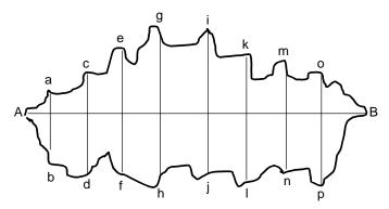
Area of irregular shape =  $L \times Z$ , where L = the distance AB, and Z = the average of the lengths measured perpendicular to AB (the sum of ab, cd, ef, etc., divided by the total number of perpendicular lengths measured; in this case, 8).
