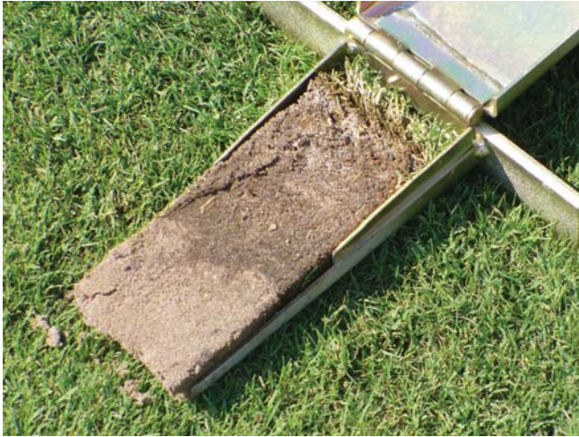
5. Core pulled from an athletic field to examine thatch buildup
